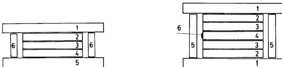
Fig. 1. Schematic diagram of the structure of an ultra-thin lithium battery: (1) anode current collector; (2) anode lithium; (3) isolator; (4) cathode film; (5) cathode current collector, and (6) glue.
